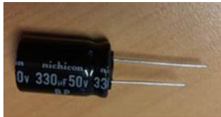
Fig. 20: Sounder End of Line Capacitor
